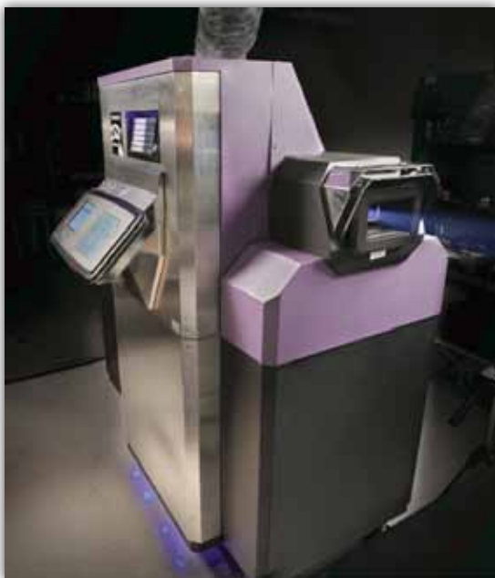
Kodak prototype laser illuminated digital cinema projector. Courtesy of Kodak, Inc.
