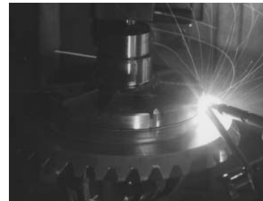
A laser welding process of a gear part is just one of Fraunhofer's many capabilities and research areas.
